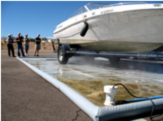
Portable decontamination pad. Lake Mead
