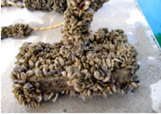
A concrete block and rope used for mussel monitoring at Lake Mead Marina covered with quagga mussels.
