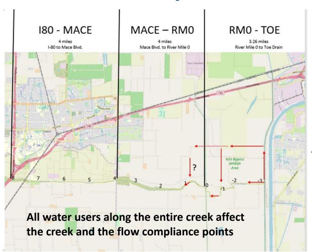
Flow direction In Summer (Red arrows), shows when Putah Creek is used for Conveyance and Wheeling
